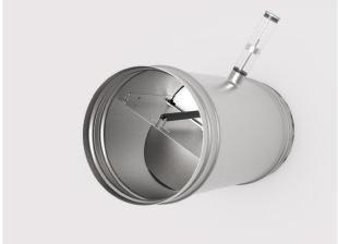
**USAGE AREA AND FEATURES :**It offers easy and economical solutions in systems where constant air flow will be used. Easily adjusted Cav dampers mechanically keep the air flow to the desired value by means of a spring. Thanks to its mechanism, it fixes its position against the changing air flow at the desired flow. In case of changing channel pressure, it prevents the change of flow by increasing or decreasing the pressure loss.
